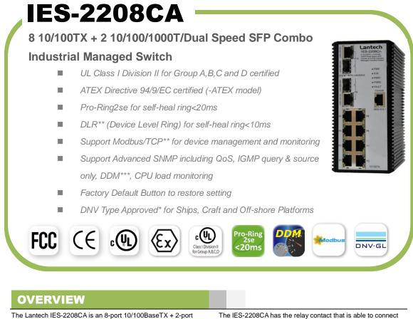
The Lantech IES-2208CA is an 8-port 10/100BaseTX + 2-port 10/100/1000T/Dual Speed SFP Combo industrial switch with Pro-Ring2se self-recovery scheme in 20ms. The SFP connection is suitable with 100M or 1000M Dual Speed. The advanced SNMP management features include QoS for 4 queues, 802.1q VLAN, IGMP snooping, query and source only for multicast IP surveillance, DDM\*\*\* as well as Web Ping,CPU load monitoring, SNTP and SMTP etc.
