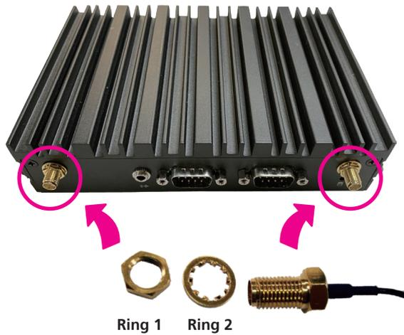
3. Connect the external antennas to the Wi-Fi antenna jacks.
