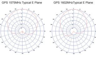
3D patterns simulated in CST microwave studio on a ground plane without cable loss.
