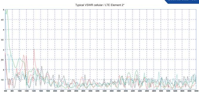
\* Red VSWR measured on a 600 x600mm (2' x 2') ground plane without extension cables | Green VSWR measured in free space without extension cables. | Blue VSWR measured in free space with 3m (10') extension cables | Black VSWR measured on a 600 x600mm (2' x 2') ground plane with 3m (10') extension cables
