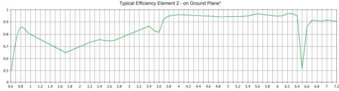
\*Efficiency simulated in CST Microwave Studio on 600x600mm (2'x2') ground plane without cable loss.
