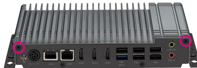
2. Once the screws are removed, lift the cover up and out of the chassis.
