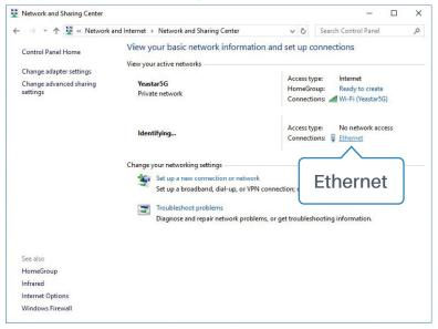
2. Go to "Properties"  $\rightarrow$  "Internet Protocol Version 4(TCP/IPv4) "and select "Use the following IP address", then assign a static IP manually within the same subnet of the gateway.
