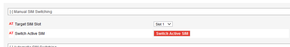
Figure 4-7: ACEmanager: WAN/Cellular > Cellular > General (Dual SIM settings)
