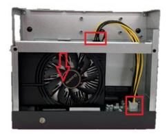
Note: The graphics card power cable will be needed when the graphics card power is over 75W.
