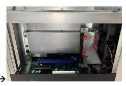
**Step 10** Align the T4 card with the slot, press the card into the slot until it is firmly seated, and screw the T4 card bracket and slot bracket to the chassis.
