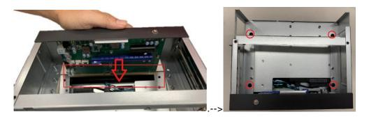
**Step 6** After installing the expansion box kit, close the system cover back to the chassis and fasten the screw. Installation is complete.
