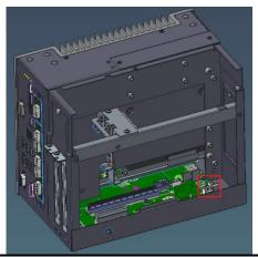
External fan module is installed.
