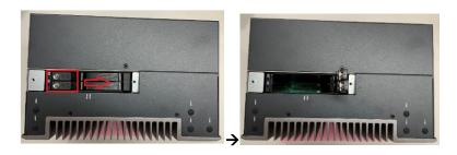
**Step 5** Align the connector of the HDD/SSD with the SATA slot of main board. Then, insert the HDD into the HDD tray.
