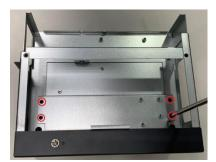
**Step 6** Screw the fan module into chassis and plug in the fan connectors.
