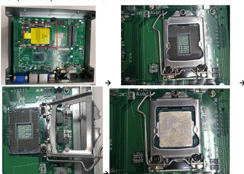
**Step 5** Apply thermal grease on top of the CPU.
