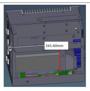
Note: Please note that 165mm of the 2<sup>nd</sup> slot is the maximum length for add-on card with I/O bracket. considering heat dissipation potential, a space of 5mm must be kept between the add-on card and T4 fan bracket.
