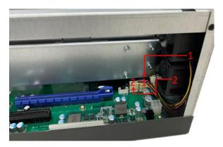
Step 7 Route the cables and put the cables in red mark area, as illustrated below.
