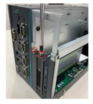
**Step 11** Insert the air duct bracket's metal part as marked B below and screw the 4 screws.
