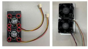
**Step 4** Paste the 4 poron pads on air duct brackets, as illustrated below.
