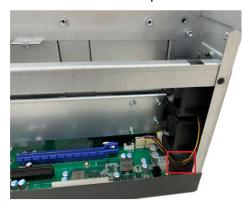
Step 8 Remove the slot brackets.
