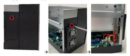
Step 6 After installing the fan module, close the system cover back to the chassis and fasten the screw. Installation is complete.
