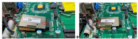
**Step 7** Paste the other thermal pad on top of the module, as illustrated below.
