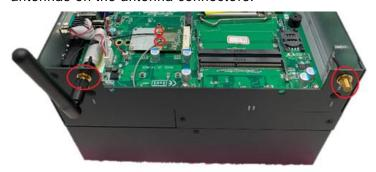
Step 7 Close the cover back to the chassis and fasten all screws. The installation is complete.
