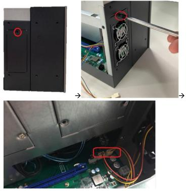
**Step 6** After installing the fan module, close the system cover back to the chassis and fasten the screw. Installation is complete.
