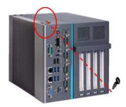
**Step 5** Insert the wireless LAN card into the slot and push it down firmly. Then screw the card tightly to the mainboard
