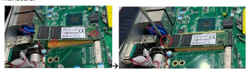
**Step 7** Paste the other thermal pad on the module and then remove the protective film, as illustrated below.
