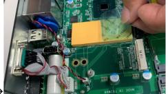
**Step 6** Insert the SSD card to slot and push it down firmly. Then screw the card tightly to the mainboard.
