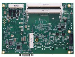
The CAPA840, a 3.5" board, supports Intel<sup>®</sup> Atom<sup>™</sup> E3845/E3827 processors. Meanwhile CAPA843, a 3.5' board, supports Intel<sup>®</sup> Celeron<sup>®</sup> J1900 processors. Both of them deliver outstanding system performance through high-bandwidth interfaces, multiple I/O functions for interactive applications and various embedded computing solutions.
