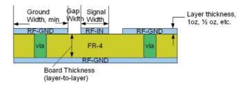
For a two-layer FR4 PCB design with 1.6mm thickness, 4.6 dielectric constant, and 1oz copper the RF-input trace should be 31mil in width, the gap to the adjacent grounds should be 6mil, and each of the RF grounds should be at least twice the width of the input signal trace (62mil). Freeware program such as AppCAD can be used to calculate values required for other configurations.
