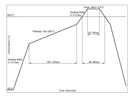
The reflow profile shown above should not be exceeded, since excessive temperatures or transport times during reflow can damage the module. Cooling temperature fall rate: max  $3^{\circ}$  / sec
