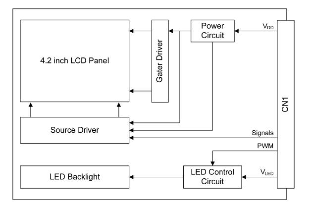
Note 1: Signals are a DEN, VD, HD, NCLK and RGB data bus.
