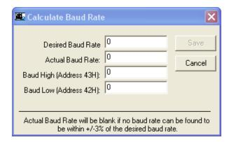
To calculate the settings for a particular baud rate, type that baud rate into the Desired Baud Rate text field. If the number in the Desired Baud Rate text field is  $\pm 3\%$  of an acceptable baud rate, the rest of the fields in the Calculate Baud Rate will automatically populate. If the baud rate is not supported by the radio, the remaining text fields will continue to display the number 0.
