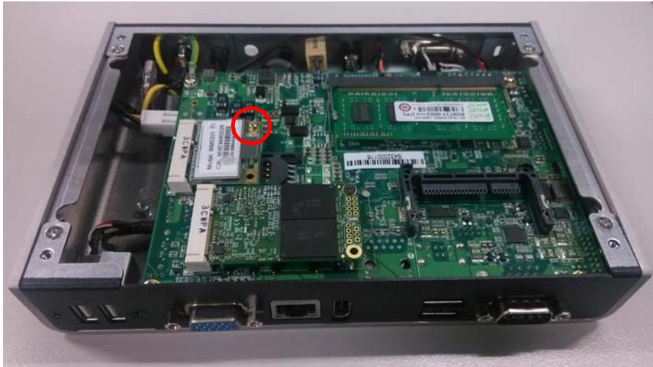
**Step 4** Find the Antenna cable and connect it with wireless LAN card.
