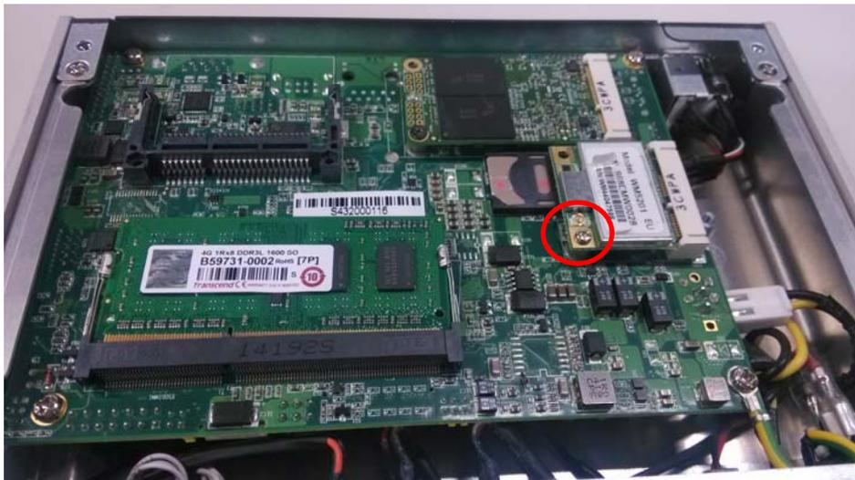
**Step 6 Find the Antenna cable and connect it with 3G module.**
