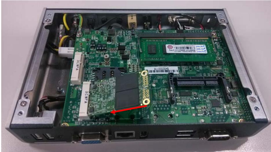
**Step 2** Push the module down, until it is firmly seated by locking two latches on the sides, and then fix the mSATA with screws with image illustrated
