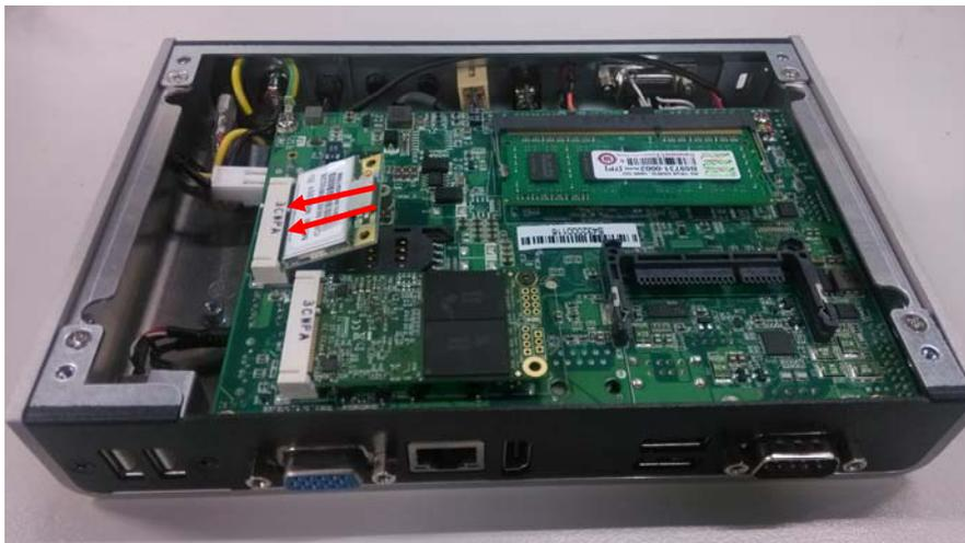
**Step 3** Press it firmly down until it is fully located and then fasten the screw per illustrated.
