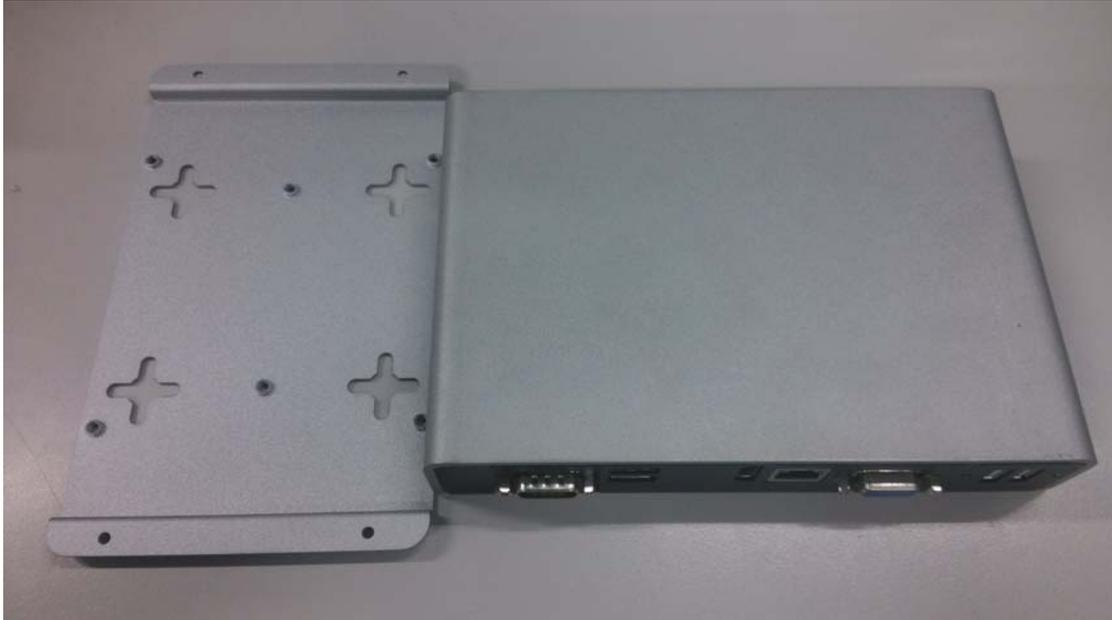
**Step 2 After loosening the screw of four footpads at the bottom of DSB320-842, and then put the DSB320-842 under VESA mount kit.**
