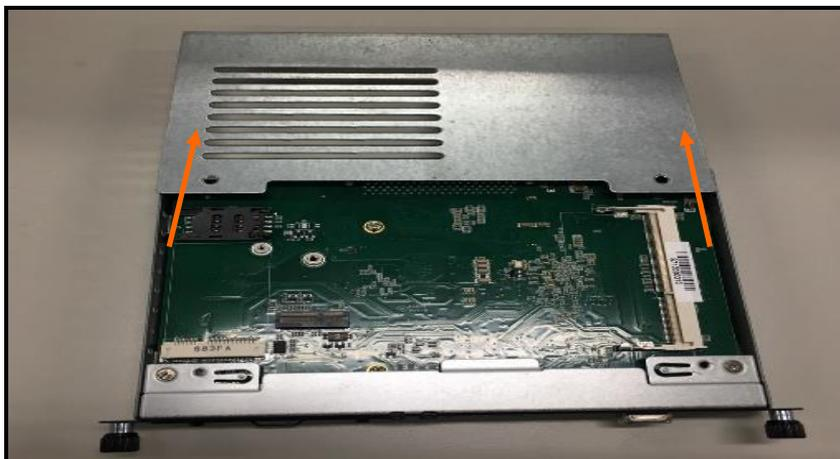
**Step 3** Please find the position of Mini PCIe & M.2 connectors on the bottom side of OPS.
