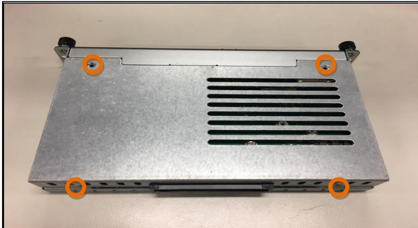
**Step 2** After losing the screws, extract the real of chassis out of the module carefully.
