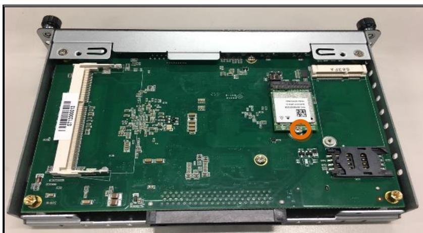
Please notice that SCN1 is one SIM slot socket and suitable to let users insert SIM card for 3G/LTE communication through mPCIe connector.
