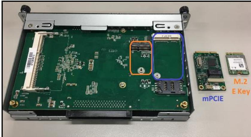
**Step 4** Please insert the mPCIe module then fasten M2X3 screw carefully.
