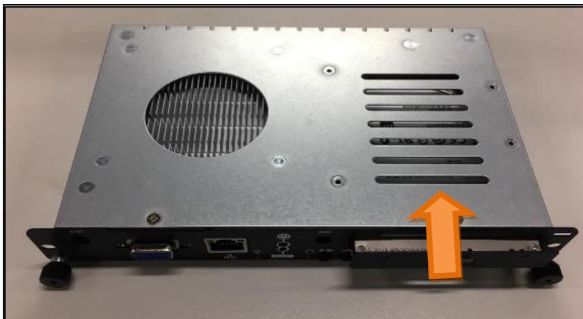
**Step 4** Finally, fasten two screws on HDD cover firmly to complete installation.
