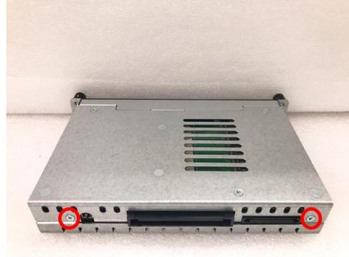
**Step 2** Slide the bottom chassis out of the module, and locate the SO-DIMM socket on the board.
