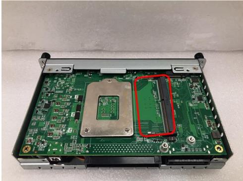
**Step 3** Place the memory module into the socket and press it firmly. The socket latches are levered upwards and clipped on to the edges of the SO-DIMM.
