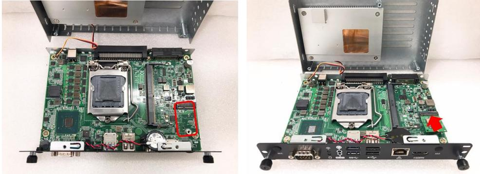
**Step 4** Then secure the M.2 2230 Key E Wi-Fi Module to the carrier by tightening up the one M3\*4L pan head screw to the marked position.
