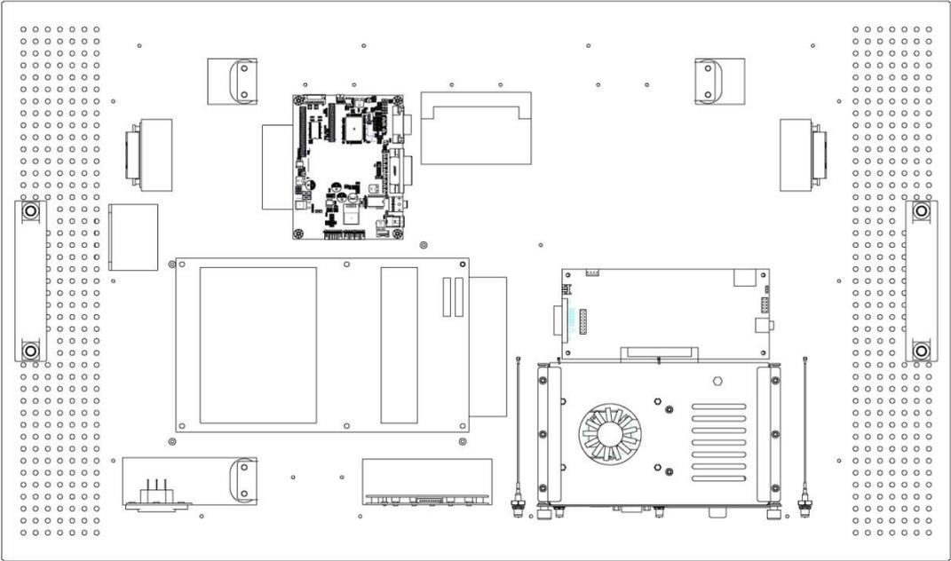
The digital signage OPS500-520-H Series prototype is based on a **32”** display panel with the functional blocks illustrated. It is mainly a 3-board partitioning design consisting of the pluggable module, docking board and the panel control board.
