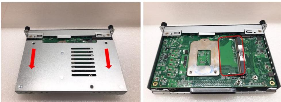
**Step 3** Place the memory module into the socket and press it firmly. The socket latches are levered upwards and clipped on to the edges of the SO-DIMM.
