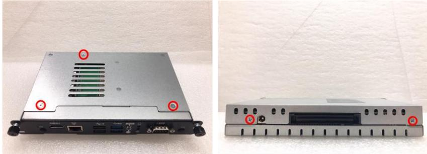
**Step 2 Slide the bottom chassis out of the module, and locate the M.2 2280 Key M slot on the board.**
