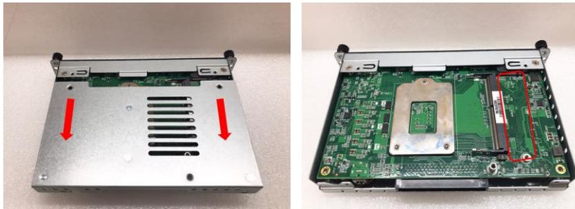
**Step 3 Holding the M.2 2280 Key M SSD card at a 30 degree angle up from horizontal, slowly insert the golden fingers into the M.2 2280 Key M slot until it is fully inserted in. And secure the M.2 2280 Key M SSD card to the carrier by tightening up the one M3\*4L pan head screw to the marked position.**
