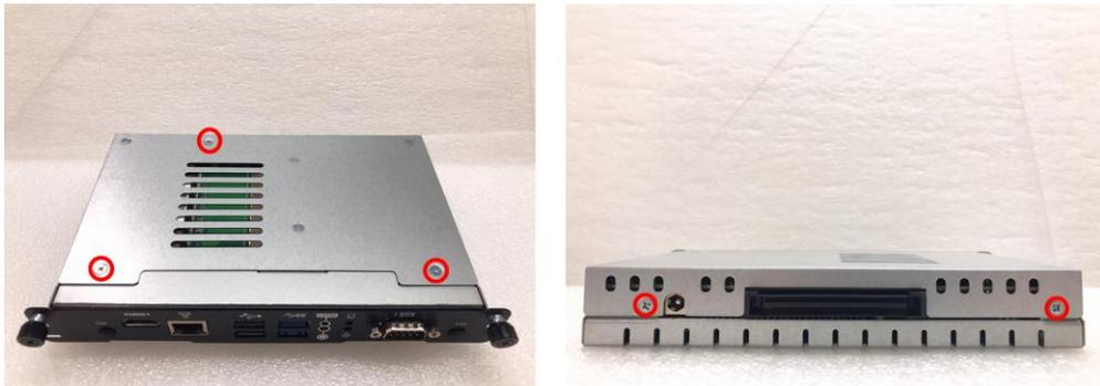
**Step 2** Slide the bottom chassis out of the module, and locate the SO-DIMM socket on the board.
