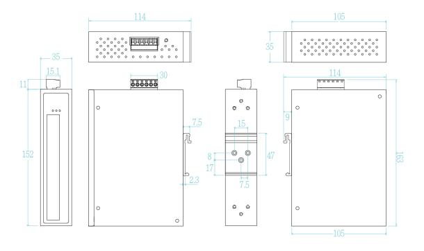
The dimensions of IPGS-0008B/IPES-0008B are  $43 \times 152 \times 105$  mm (W x H x D). The figure below gives the dimensions and views of each side of the 8-port 10/100/1000Base-T Industrial Switch.
