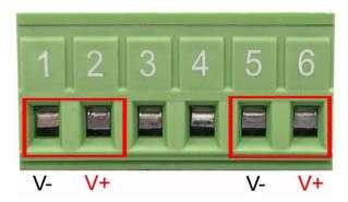
Insert the positive and negative wires into the V+ and V- contacts on the terminal block connector.
