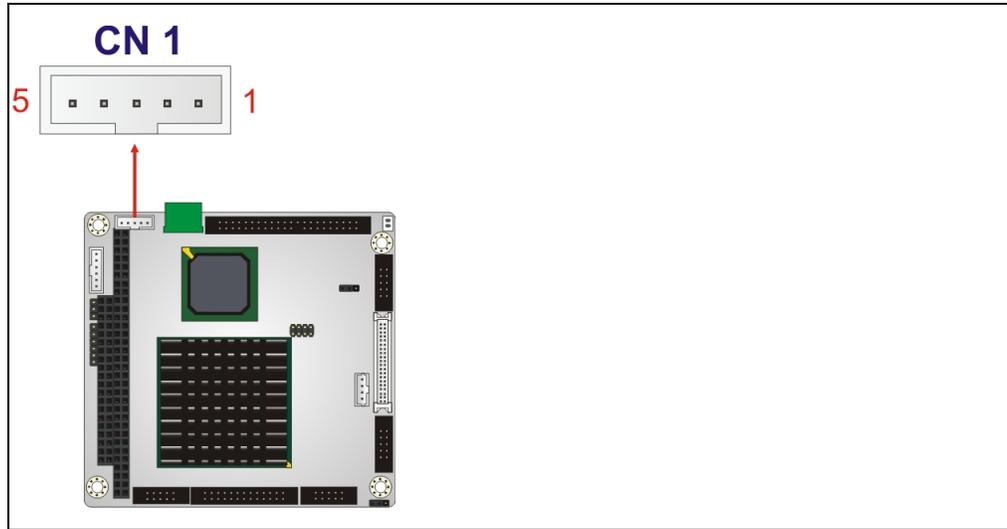
**Figure 3-12: LCD Inverter Connector Location**
