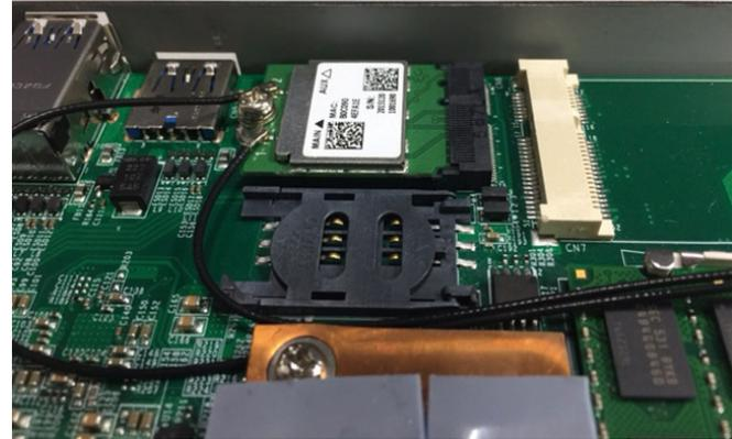
5. Insert the antenna jack end of the cable through the antenna hole.
