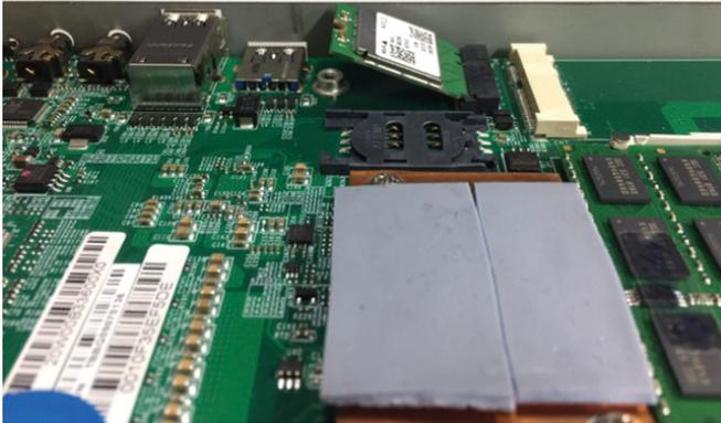
4. Secure the module with mounting screws and attach one end of the RF cables onto the module.
