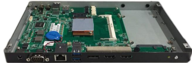
3. Insert the NGFF M.2 Wi-Fi module into the NGFF M.2 slot at a 45 degree angle until the gold-plated connector on the edge of the module completely disappears inside the slot.
