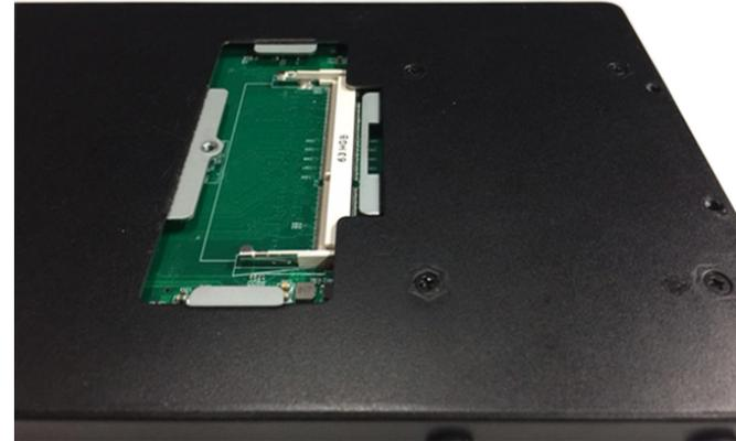
4. Insert the module into the socket at an approximately 30 degrees angle and then push the module down until the clips on both sides of the socket lock into position.
