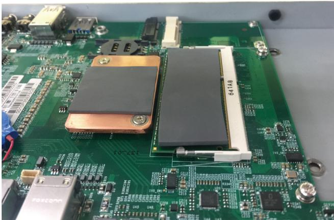
3. Open the bottom cover for installing the 2nd SO-DIMM memory module.
