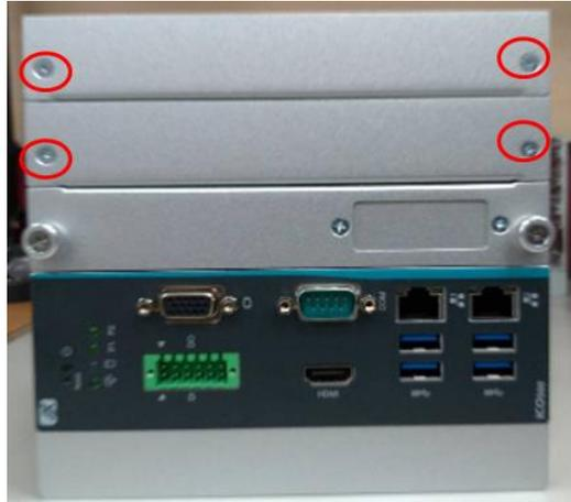
**Step 3** Install the module card as shown below, and fasten the screws firmly to finish the installation.
