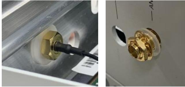
**Step 4** Hold the other side and screw the antenna.
