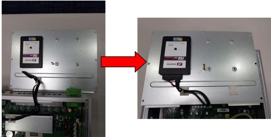
**Step 6 Put the bottom cover and fasten all the screws back onto the system.**
