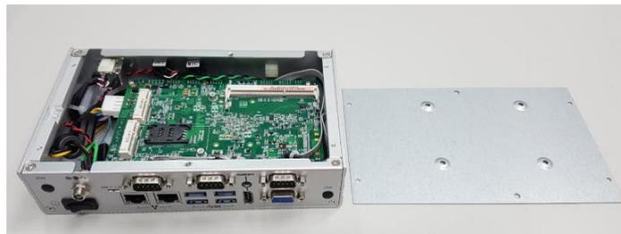
**Step 4** Locate the DDR3L SO-DIMM slot, holding the DDR3L SO-DIMM at a 30 degree angle up from horizontal; slowly insert the golden fingers into the DDR3L SO-DIMM slot until it is fully inserted in.
