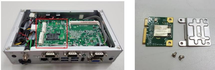
**Step 5** Holding the Wi-Fi PCI Express mini card at a 45 degree angle up from horizontal; slowly insert the golden fingers into the PCI Express slot until it is fully inserted in and fasten screws and connect the cable to antenna.
