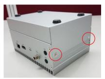
Step 3 Remove the bottom cover (notice the direction mark) and HDD cover.
