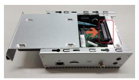
Step 8 Recover the bottom cover and fasten two screws on the side of the system.
