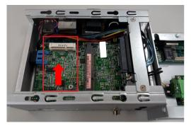
Step 5 Slide Mini Card into Mini Card slot with caution, and fasten screw of Express Mini Card.
