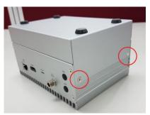
Step 3 Remove the bottom cover (notice the direction mark) and HDD cover.
