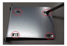
Step 7 Connected the SSD/HDD directly and make sure the insertion is complete.
