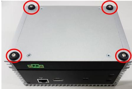
**Step 3** Loosen the screws to remove SSD/HDD bracket then a SO-DIMM socket on main board is visible.
