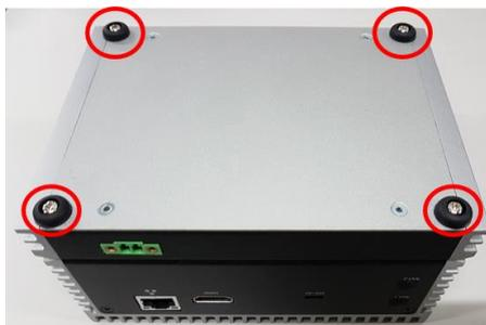
Step 3 Loosen the screws to remove SSD/HDD bracket and then located the Mini PCIe slot.
