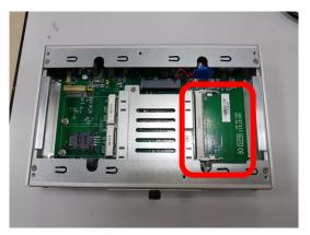
Step 4 Locate the memory module, insert a gold colored contact into the socket and push the module two end latches till locked.
