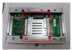
Step 5 Before assemble the SSD/HDD, please loosen the thumb screw to remove the HDD bracket, and then assemble the SSD/HDD with the one HDD mounting screw.
