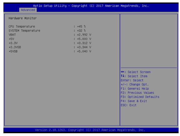
This screen displays the temperature of system and CPU, system voltages (VCORE, +3.3V, +12V and +5V).
