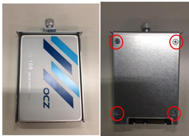
Figure 2-5 Fasten the four screws
