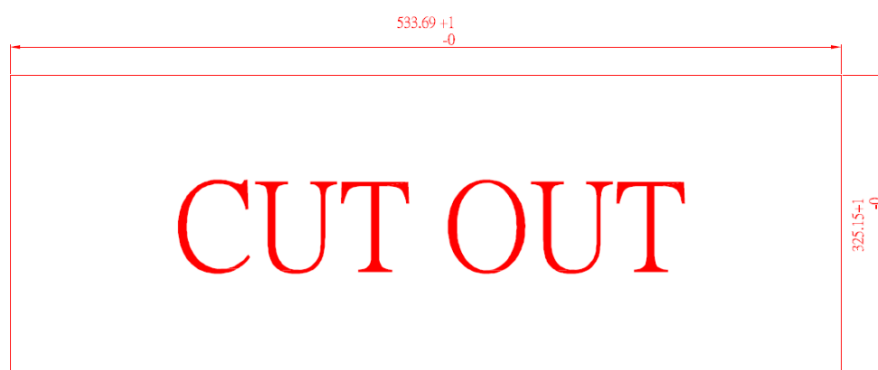
Diagram 1-3 Cutting-out dimensions of the GOT321W-502-PCT
